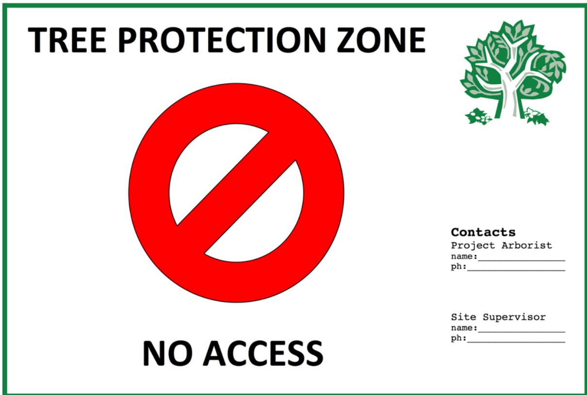
Example of Tree Protection Zone signage
